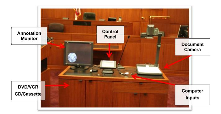
**Control Panel** – The controller for components used to project evidence; it also contains functional buttons for controlling the evidence presentation system.
